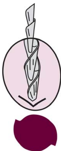
Fig. 8.7: Cross-section and longitudinal shape of S-file
